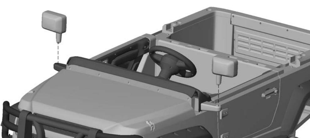
C. Fix 2 rear view mirrors by install them onto right position.
