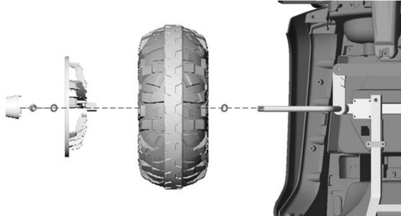
A. Assemble the front bumper firstly by putting shim, wheel, bushing, shim, wheel cover, and fix it by screws;
