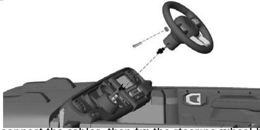
Install the steering pole, and connect the cables, then fix the steering wheel by screws.
