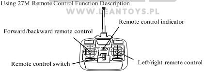
The installation of remote antenna: screw the remote antenna in the remote control clockwise.
