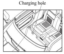
Plug the charger into the electric outlet; Insert a port of the charger into the charging hole below the seat cushion.
