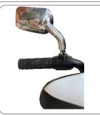
Install the mirror: align the mirror with the body Press firmly on it;
