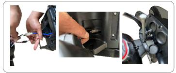
Install the front: first connect the front with Body line connection, plug the head Into the hole, stuck on the body, Tighten with long screws as shown Just
