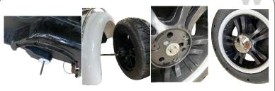
Install the rear wheel: put the rear axle through Into the body. Put the rear wheel in The rear axle clamps the gasket clip , And finally fasten the wheels can;
