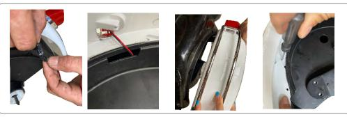
Install the rear mudguard: first connect the mudguard line with the body line, the excess line is inserted into the hole and stuck in the body Tighten with screws;
