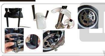
Install the front wheel: remove the front axle Press the front tile, and the front fork guard Use screws to tighten the left and right Black plastic parts aligned on the front wheel Hole position as shown in the figure, tighten the screws That's it!
