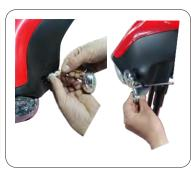
Install the turn signal: connect the turn signal line with Body line docking. Tighten with screws
