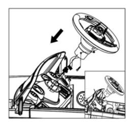
•Connect the terminal of the steering wheel to terminal of the instrument panel , put the wire back to instrument panel if they are too long.
