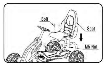
As showed in the picture,install the seat to the corresponding place, and fasten with the bolt and nuts.
