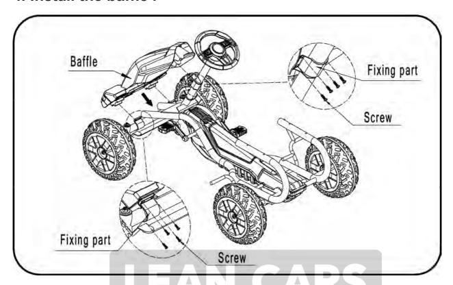
As showed in the picture,install the baffle to the corresponding place, and fasten with the fixing part and screws.
