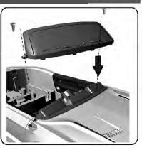
**5. Install the reflector** Insert the mirror directly into the body.
