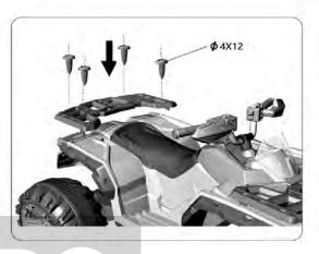
• Install the rear frame directly with 4 screws to the body
