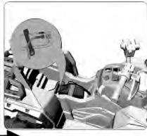
• First, remove the seat cushion with a screwdriver and insert the red plug into the red end of the battery and cover the seat with screws
