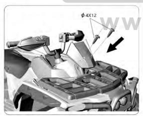
• Put the windscreen in the front of the instrument, align the screw hole, and fix it with 2 screws
