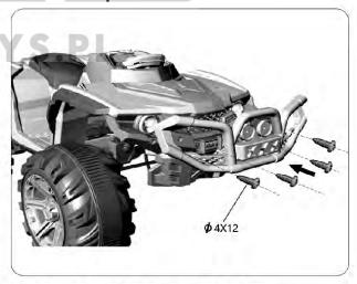
Fix the front bumper directly to the body with screws
