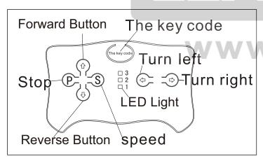
The remote control operation always prior to the foot pedals operation.(The foot pedal won't work whileoperating remote control)
