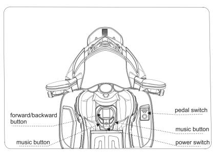
power switch and forward/backward switch are on the front part of the car Power switch Press the power switch to open, it will turn off if press again
