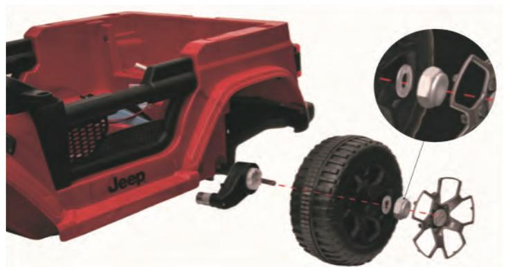
Please install motor, wheel, bushing, gasket, nut, wheel cover following the sequence. (No need bushing when install EVA wheels)
