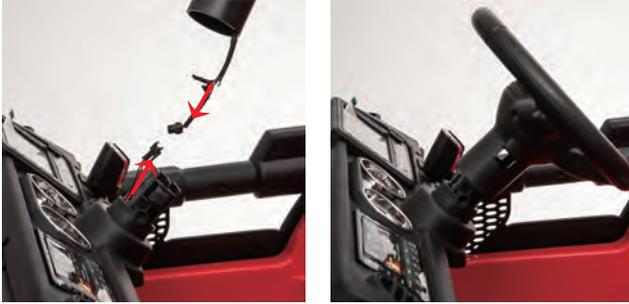
Connect power line first, and then assemble the steering wheel by pressing it down directly.
