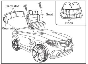
7.Assemble the empennage and seat cushion buckle into the body corresponding to the position ,fix the snap with the neck on the car body, then fasten by reoccupy two selftapping screws
