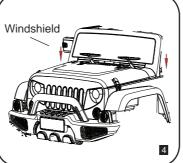
Mounting windshield ne windshield is taken out, then the vehicle vindshield card angular alignment groove, pressed down hear clicks that place. (as shown in figure 4)
