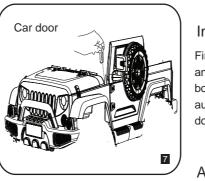
First, the distinction between left and right door and door mirrors, and then into the corresponding body, followed by three T4.0\*16 large flat head automatic screw the lock, finally will mirror into the door or not installed anti. (as shown in Figure 7)
