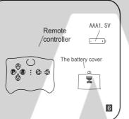
First use the screwdriver to unscrew the screw on the battery cover, then take out the battery cover and remote control into two AA1.5 V batteries, and battery cover cover and screw
