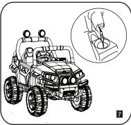
Install the rear spotlamp bracket First, connect the connector on the assembled rear bracket with the plug-in on the vehicle body, then put the wire and plug-in into the hole, and then align the rear spotlights with the vehicle body card slot, with a total of 4 card slots at the front, rear, left and right, and press down hard to hear the click sound, which indicates that it is installed in place. (As shown in figure 7)
