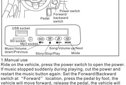
stop. Set the Forward/Backward switch at "Backward" location, press the pedal by foot, the vehicle will move backward, release the pedal, the vehicle will stop. Set the Forward/Backward switch at middle location, press the pedal by foot, the vehicle won't move. 2.Remote control use Ride on the vehicle, press the power switch to open the power. If music stopped suddenly during playing, cut the power and
